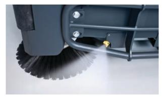
Patented DustGuard™ is proven to reduce airborne dust generated by side broom sweeping. An ultra fine fog suppresses fugitive dust.
