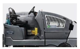
The CS7020 has a fully adjustable seat (with built-in arm rest and seat belt) and tilt steering.
